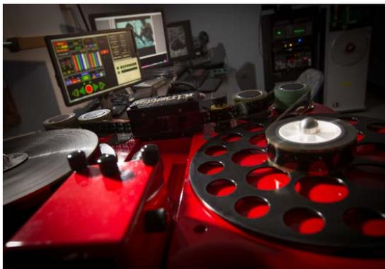
Based on the film type and gauge and the desired file output, our engineers select the scanner that best suits the client's reels. We can scan all film gauges from 8mm to 35mm on any stock, with 8mm and 16mm representing the majority of our transfers. Our engineers have extensive knowledge and experience with these formats, enabling them to successfully transfer films with severe condition issues, including shrinkage and emulsion lift.
